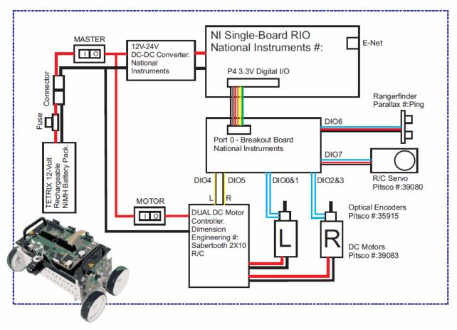
LabVIEW Robotics Starter Kit (Block Diagram)
