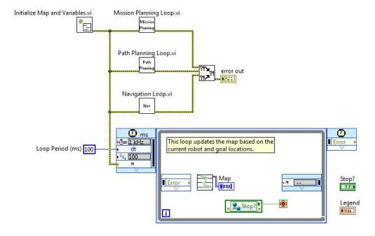
Figure 2. An Advanced Robotics Program With Multiple Subsystems Executing in Parallel
