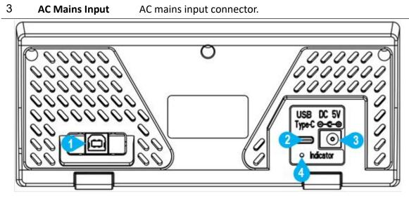
Figure 2-3 Rear panel overview (Take the AC power supply for instance)
