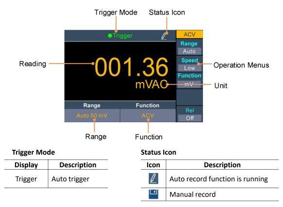
Figure 2-4 User interface (Single display - Take the model with DC power supply for instance)
