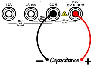
**Tip:** Please short contact the two feet of an electrolytic capacitor by using a test lead before measuring the electrolytic capacitor.
