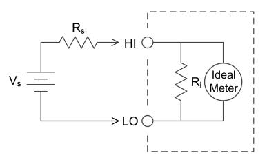
$V_s$  = ideal DUT voltage  $R_s$  = DUT source resistance  $R_i$  = multimeter input resistance
