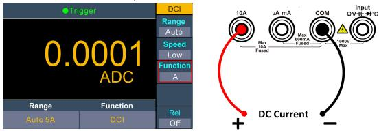
When the Function is set as mA, connect the test lead as below.
