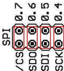
The LPC2148 microcontroller features 2 SPI interfaces i.e. SPI0 and SPI1. On LPC2148 development board SPI0 is used for interfacing SD/MMC card. The SPI expansion
