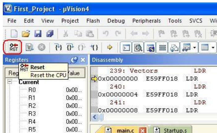
13. Observe that CCLK is also reset and now it is equal to XTAL frequency. Similarly the GPIO and pin connect block vales are also reset.
