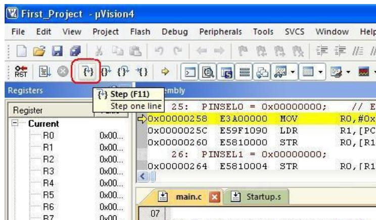
11. When you encounter the delay function you can simply use Step Out function. It will execute the delay function and take execution to the next line immediately after the delay function.
