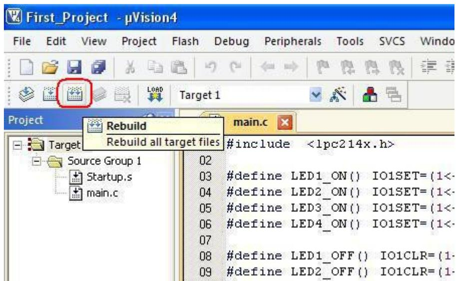
21. You can alternatively build project by clicking on **Project>Build Target** from the main menu.
