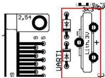
The LPC2148 microcontroller features an in-built RTC and it provides Seconds, Minutes, Hours, Day of Month, Month, Year, Day of Week, and Day of Year. It has a dedicated 32.768 kHz oscillator or programmable prescaler from VPB clock. It also has a dedicated power supply pin that can be connected to a battery or to the board supply of 3.3V. LPC2148 development board has battery holder for providing battery back up to the internal RTC.
