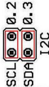
The I2C0 peripheral on LPC2148 development board is used for interfacing 24LCxxx EEPROM memories from microchip. The above figure describes the jumper positions and pins used for I2C interface.
