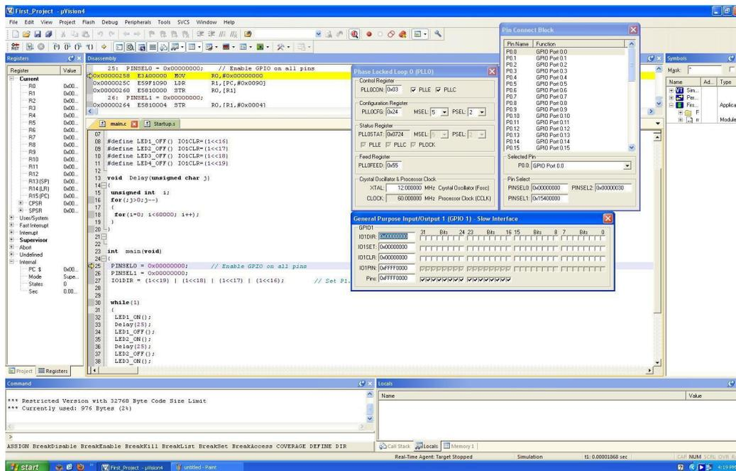
10. Now use **Step** function to step through the code. Alternatively you can press **Ctrl+F11**. Observe the changes in the Pin connect block and Port1 block as you step through the code.
