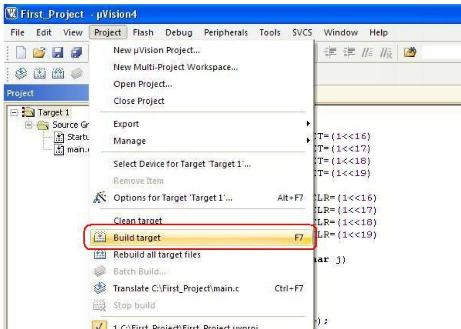
22. You can observe the build process in the output window. If any errors, rectify it by double clicking on it and you will be pointed to the erroneous line.
