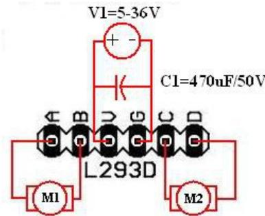
Fig.3.5 Supply and motor connections
