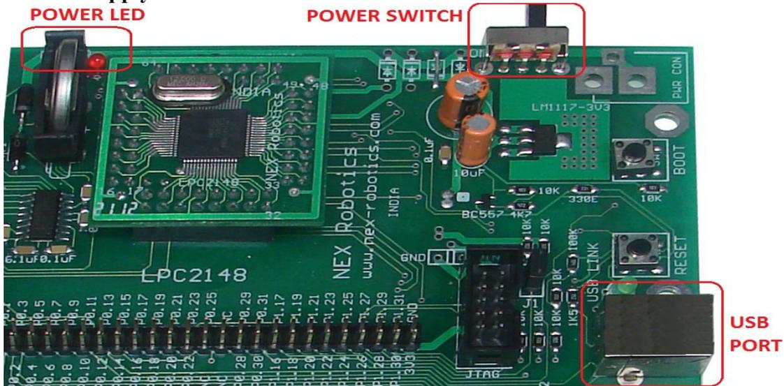
The USB powered version of LPC2148 development board is powered using USB port.
