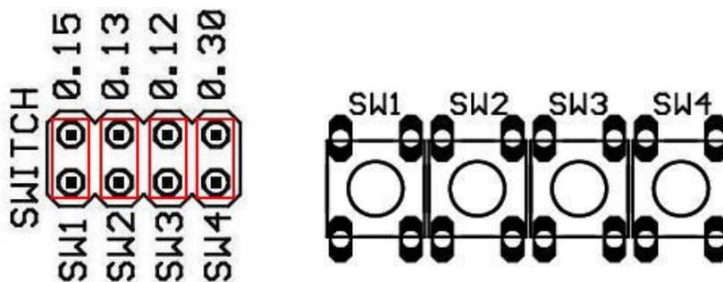
LPC2148 development board has 4 user programmable switches. The ports pins and jumper settings are as shown in the above figure. When a switch is pressed it will pull the associated pin to logic '0'. Port pins P0.15 and P0.30 features alternate function of external interrupts. Jumper SW1 is associated with switch SW1 and so on.
