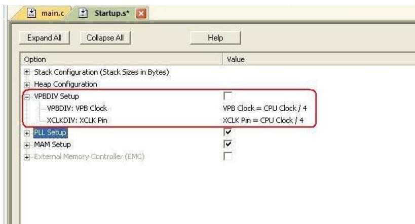
Observe that in the default mode it is not included but at reset the VPBDIV loads the default value that is  $\frac{1}{4}$  of the CPU clock. Using the configuration wizard you can set the peripheral clock as:
