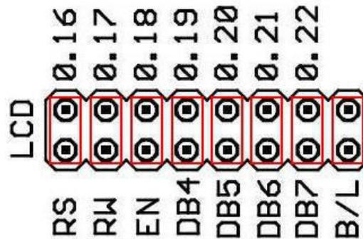
The LPC2148 development board is included with 4-bit HD44780 based LCD interface. It can be used to interface 16x1, 16x2, 20x4 characters LCD display. The board is shipped with 16x2 character LCD display. The jumper positions and port pins are as shown in the above figure. The **B/L** jumper setting is used to control LCD backlight. On removing this jumper LCD backlight will turn OFF.
