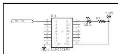
The cathode of LED is connected to the pin named as '1' on Driver header and I/O pin connected is connected to pin named as '1' on Logic header by placing a jumper in its position.
