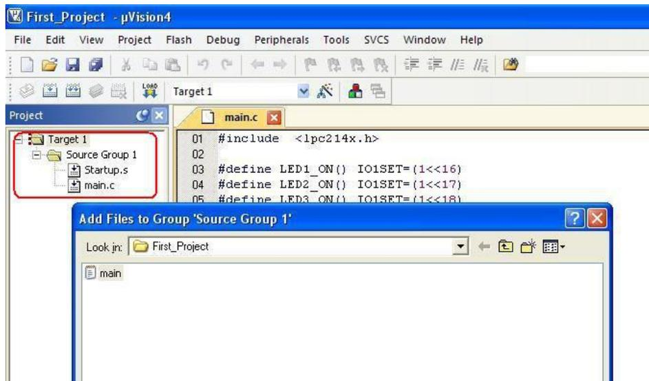
15. Right click **Target1** in the project explorer window and select the highlighted option as shown in the fig. below.
