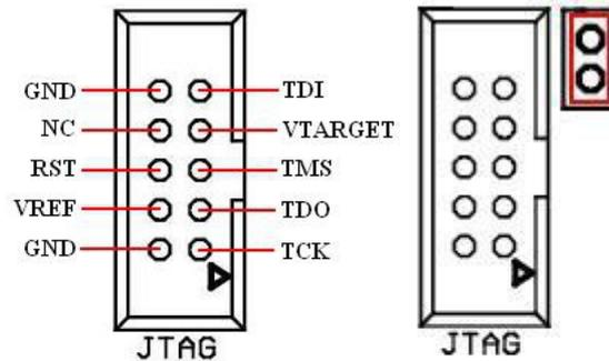
The LPC2148 development board has a 10pin (2X5) JTAG box header for on chip debugging. JTAG debugging requires pulling P1.26 low on reset in order to enter into debug mode. To achieve this there is a 2 pin jumper on the development board as shown in the figure above.
