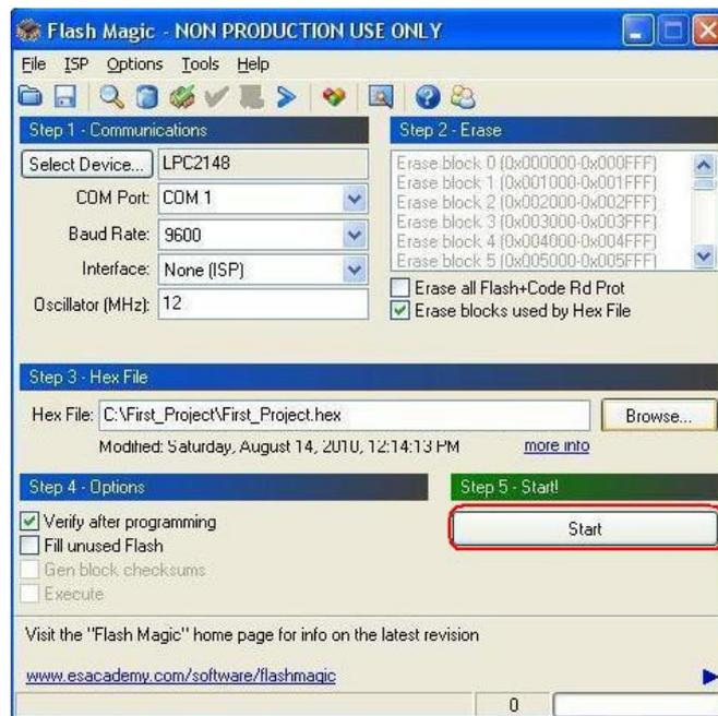
8. Observe the status bar at the bottom of the Flash Magic tool. Wait for the “**Finished**” status and press “**Reset**” on the LPC2148 development board and observe the LEDs.
