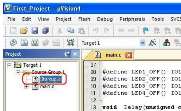
2. The startup.s file will open up as assembly file. To open the wizard click **Configuration Wizard** as shown in figure below.
