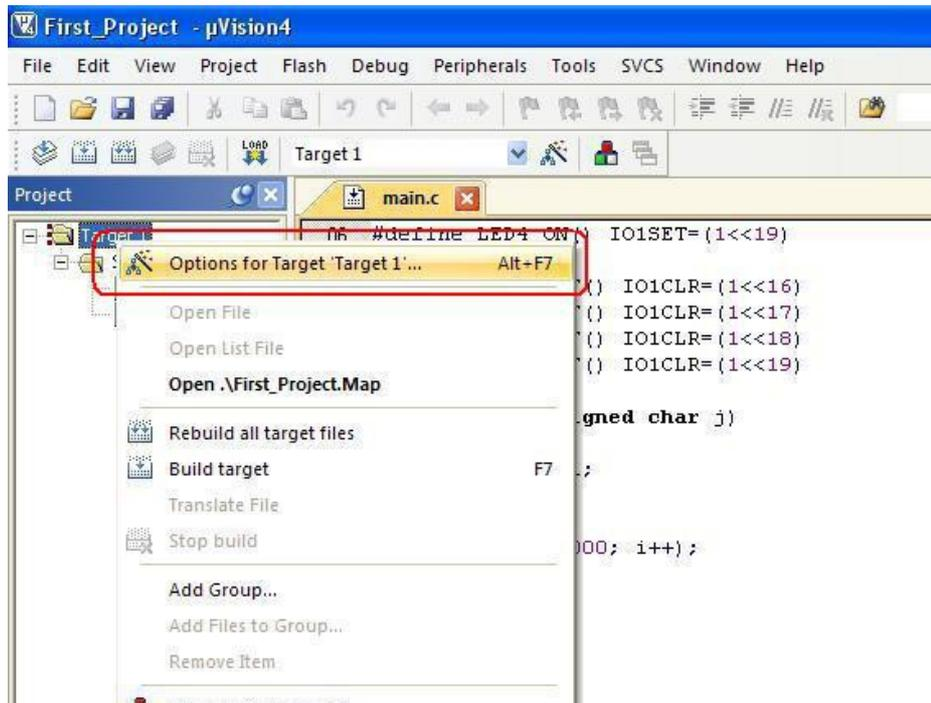
16. In the appearing window select **Target** tab and set Xtal. frequency as 12MHz.
