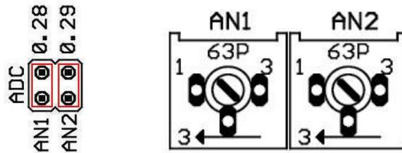
LPC2148 development board has two trimpots connected to AD0.1 and AD0.2 on the LPC2148 microcontroller. The jumper positions are as shown in the above figure. Jumper AN1 represents trimpot AN1 and AN2 represents trimpot AN2. The trimpot voltage range lies between 0-3.3V.
