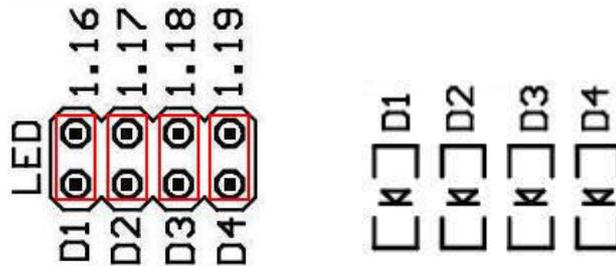
LPC2148 development board has 4 user programmable LEDs. The port pins for LEDs are as shown in the above figure. Jumper D1 is associated with Led D1 and so on. Jumper positions are as shown in the above figure. Alternatively you can make connection between any port pin and LED directly using 1to1 cables. All LEDs are common ground with series resistor of 1K.
